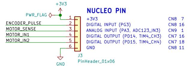
Motor driver and encoder prototype board
